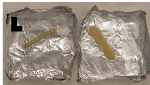
Fig. 1. PLA melted in foil trays. Coated specimen on the left.
