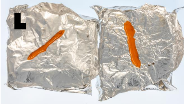
Fig. 2. PETG melted in foil trays. Coated specimen on the left.
