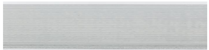
Fig. 11. Ø1.75 PC at 280 °C with a 0.8 mm nozzle
