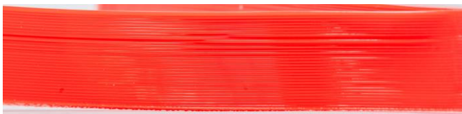
Fig. 16. Ø1.75 TPU-HF at 230 °C with a 0.6 mm nozzle
