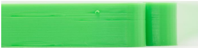
Fig. 6. Ø1.75 PETG-HF at 245 °C with a 0.4 mm nozzle
