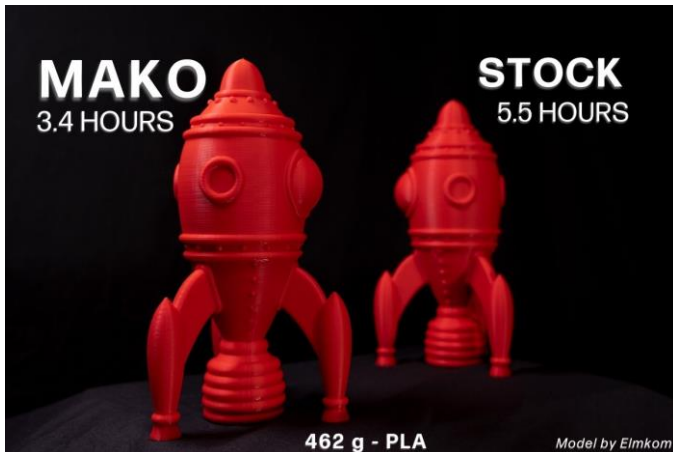
Fig. 18. Printing comparison between Mako and the stock hotend for a rocket model. The print used a 0.6 mm nozzle and Bambu Lab's PLA Basic filament.
