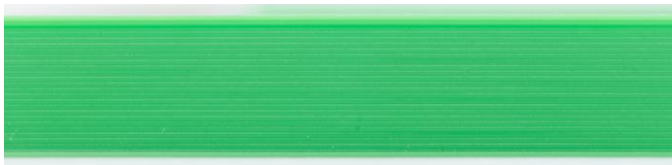
Fig. 8. Ø1.75 PETG-HF at 245 °C with a 0.8 mm nozzle
