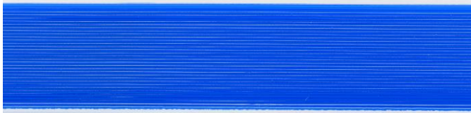
Fig. 13. Ø1.75 ABS at 270 °C with a 0.6 mm nozzle
