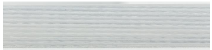
Fig. 10. Ø1.75 PC at 280 °C with a 0.6 mm nozzle
