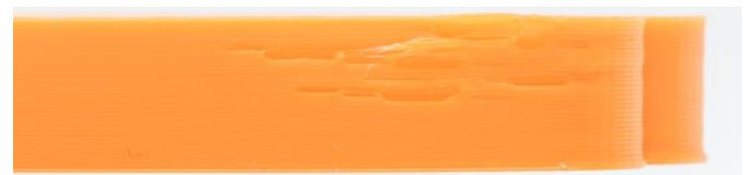
Fig. 4. Ø1.75 PLA at 220 °C with a 0.6 mm nozzle
