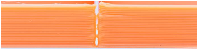
Fig. 5. Ø1.75 PLA at 220 °C with a 0.8 mm nozzle
