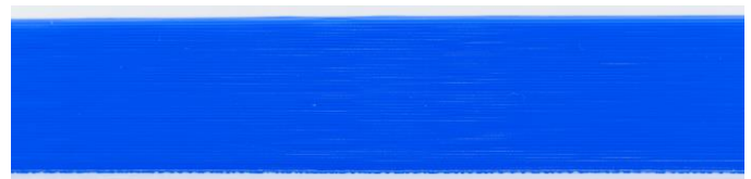
Fig. 12. Ø1.75 ABS at 270 °C with a 0.4 mm nozzle
