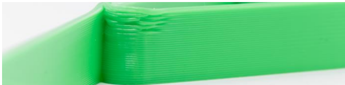
Fig. 7. Ø1.75 PETG-HF at 245 °C with a 0.6 mm nozzle
