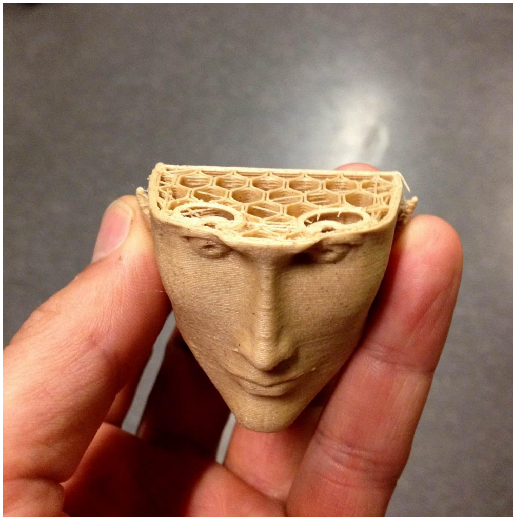
Showing the light infill pattern of the 3D printed face
