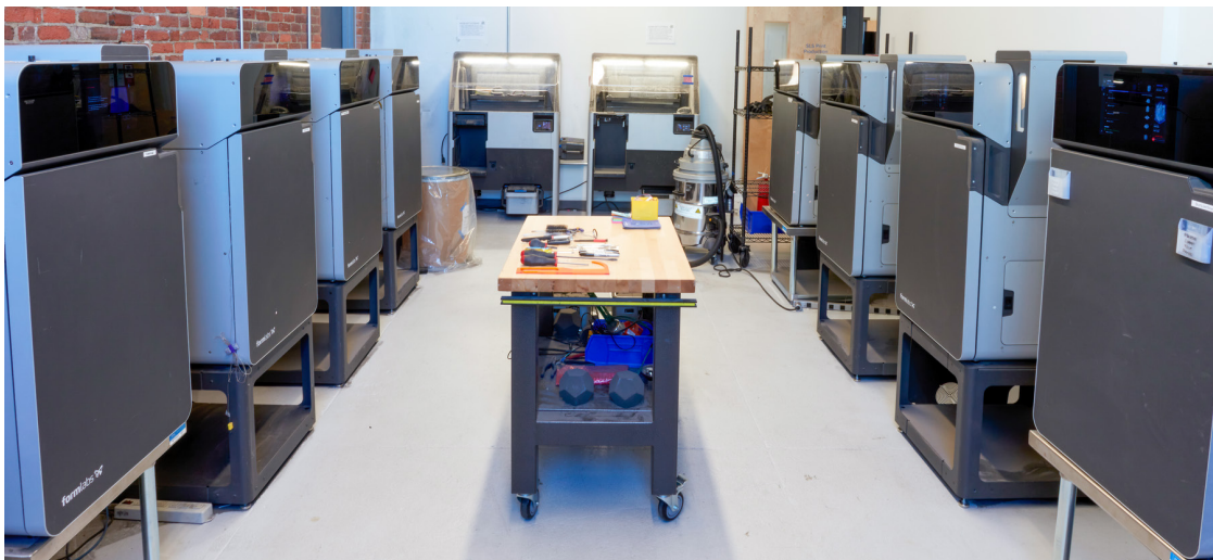
Formlabs R&D SLS materials lab in Somerville is about 37 m 2 (180 m 3 ) with over 10 Fuse printers and four Fuse Sifts.
