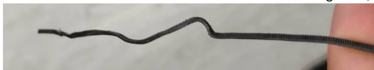
Figure 11: Filament deformation caused by soft wet filament
