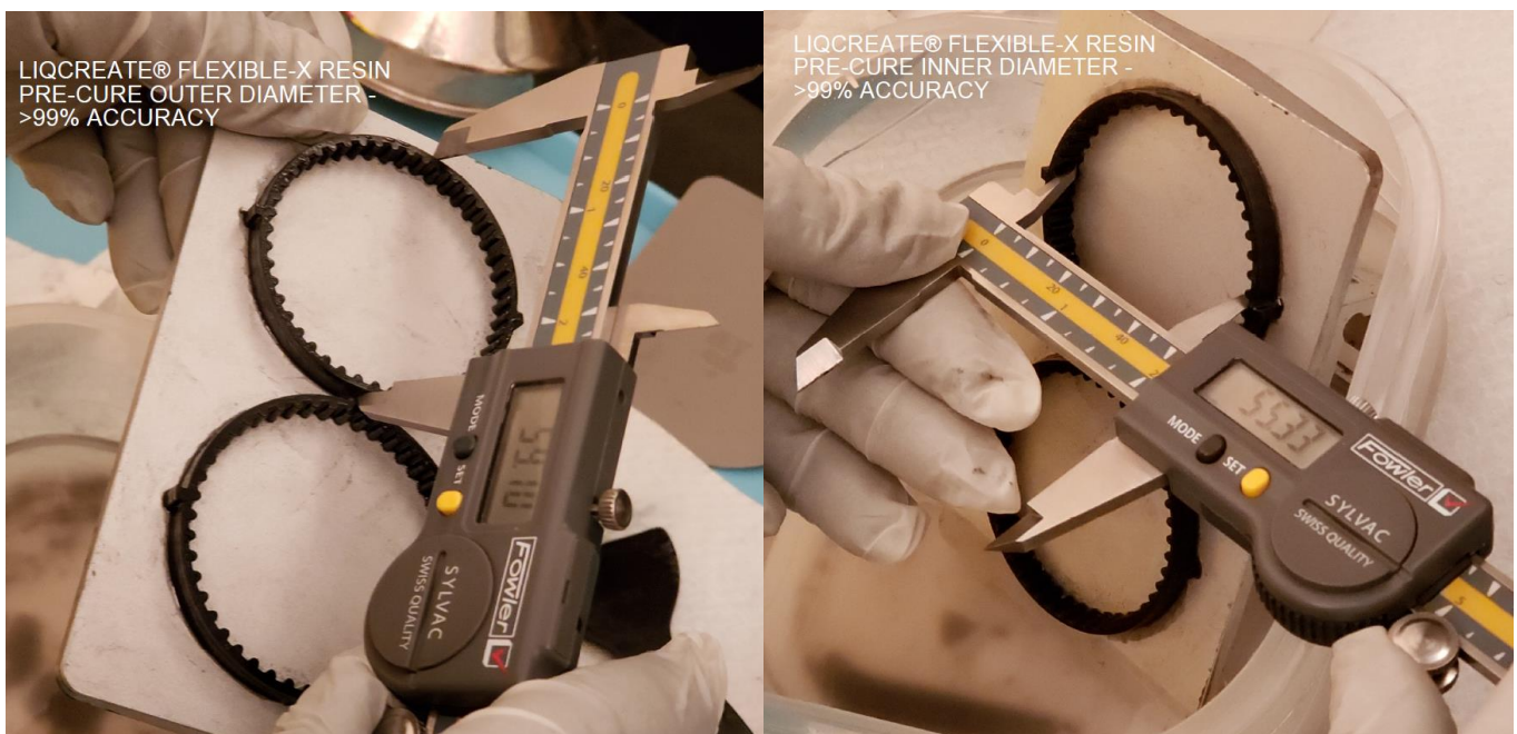
Image: Accuracy measurement of 3D-printed Flexible-X parts.
