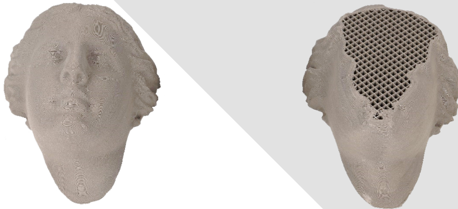
Figure 25. Mass reduction using infill
