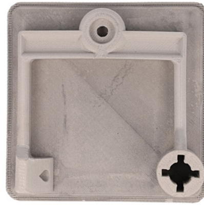
Figure 22. Use of shrinkage plate ensure uniform shrinkage
