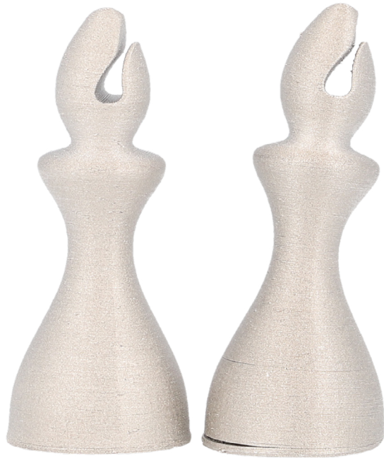
Figure 16. Warped Bottom can lead to failure
