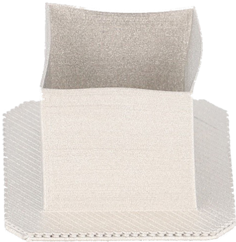
Figure 12. 0,4 mm Wall Failure
