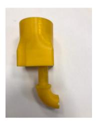
Another example is a suction system Sonmak printed to remove dust from their machine, to prevent the dust from spreading into the environment.
