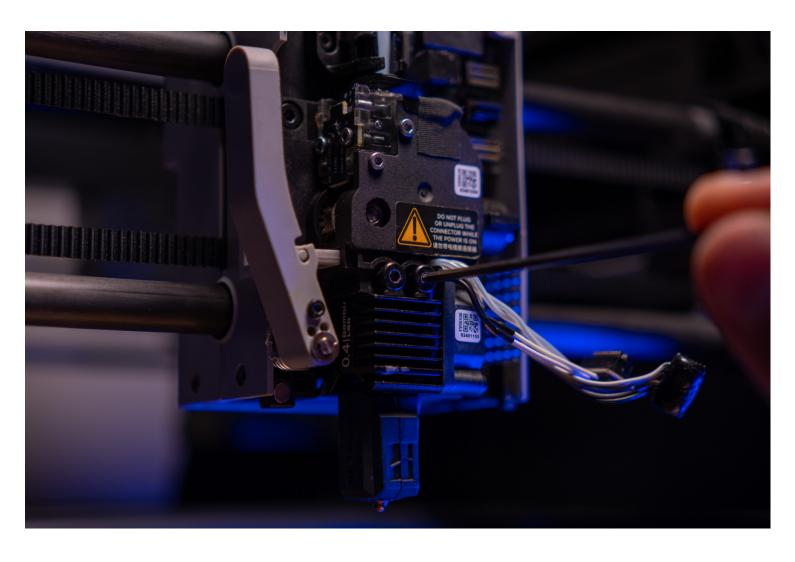
**Step 4:** Carefully and gently move the wires out of the plastic wire clip and remove the complete hotend assembly.
