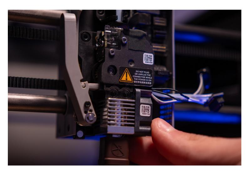
**Step 2:** Gently push the 2 screws in and then tighten them equally, be careful not to over-tighten
