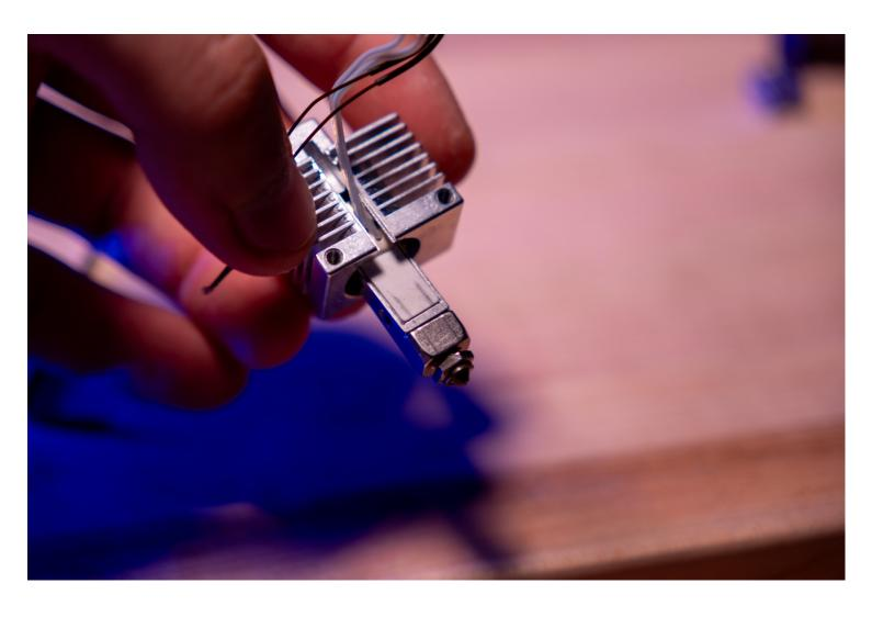
**Step 4:** Slide the retaining clip onto the bottom of the heater to hold it in place while you complete the next step.
